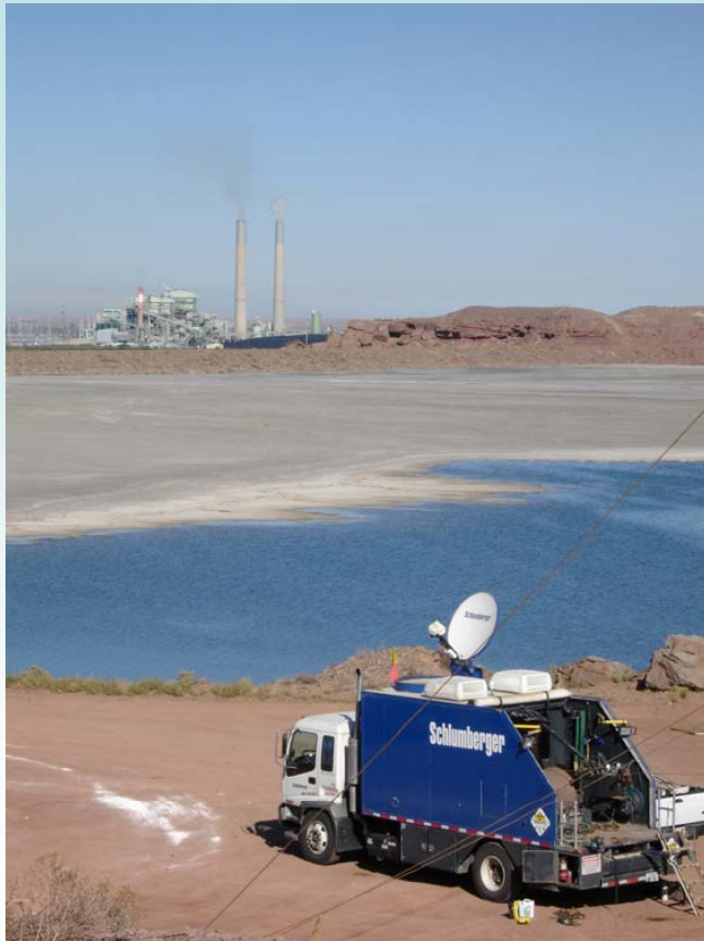
Schlumberger well log processing truck on location in Arizona (Photo: R. Trautz, EPRI)
